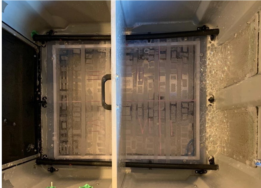
Figure 1. The euthanasia box interior with foam generators on the right side where the piglets were placed. Along the sides are the black jet pulse system and the floor is marked with red tape into four squares.
