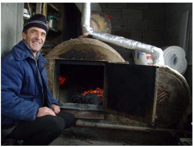
FIGURE 60: MAN IN ANTONESTI WITH A BIOMASS BURNER HE BUILT INSPIRED BY THE REAW PROJECT, PHOTO BY ANNELIE KJELLBERG
