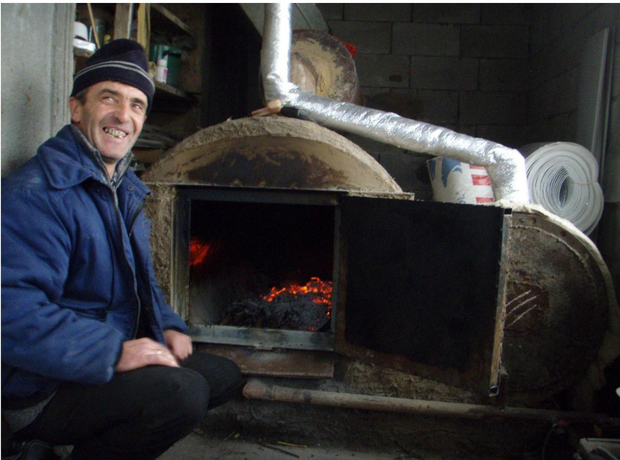
FIGURE 60: MAN IN ANTONESTI WITH A BIOMASS BURNER HE BUILT INSPIRED BY THE REAW PROJECT. PHOTO BY ANNELIE KJELLBERG
