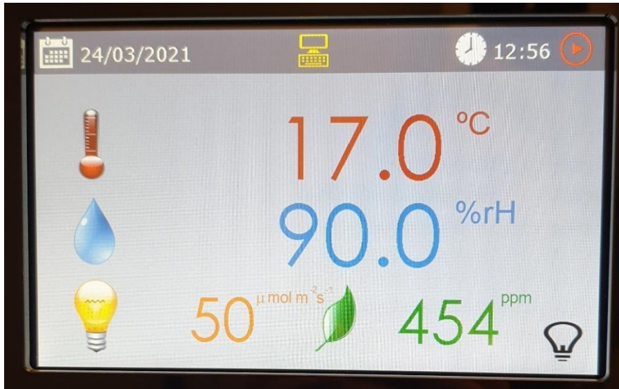
Figure 5: The screen showing the real-time conditions inside the climate chamber.
