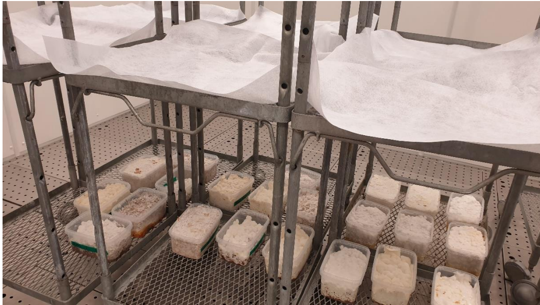
Figure 9: Boxes in climate chamber, with fibre cloth above to reduce light.
