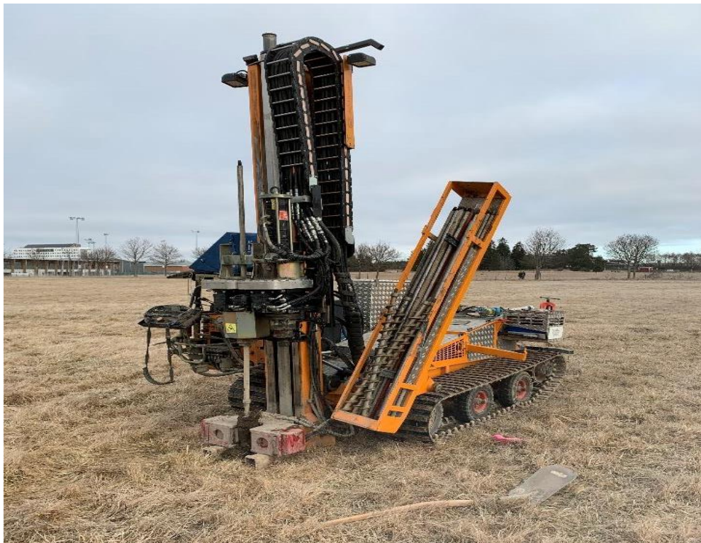
Figure 5. Screw drill machine method with drilling track
