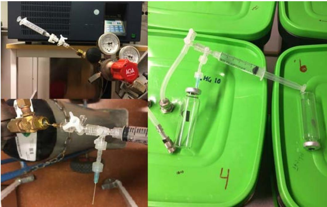
*Figure 4: Sampling during resting phase using a syringe filled with 1 atm overpressure of N<sub>2</sub> gas.*
