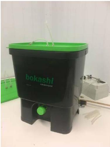
*Figure 1: Bokashi bucket installed with gas sampling devices.*
