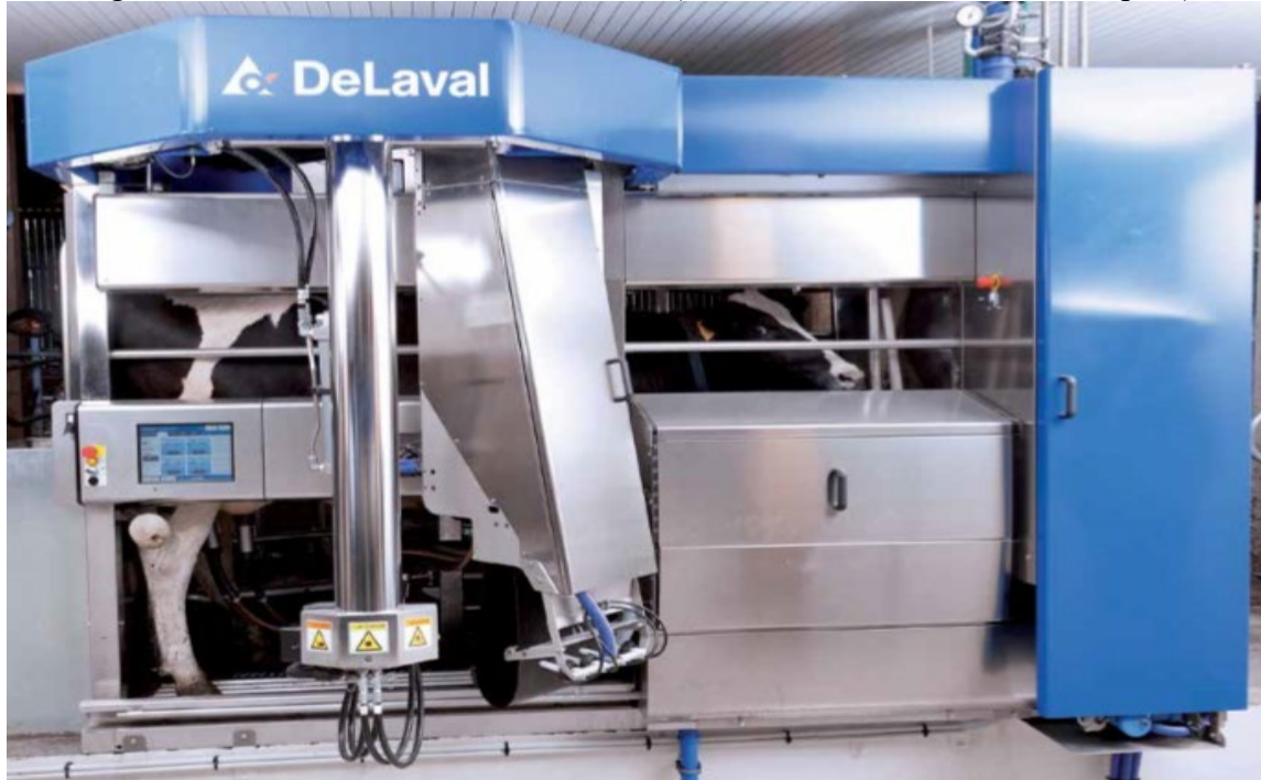
Figure 10. Typical VMS during a milking session (DeLaval_Catalogue_English, 2014, p.48).
