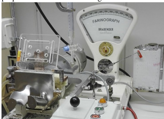
Figure I. The farinograph used in baking. The mixing blades are seen on the bottom left.
