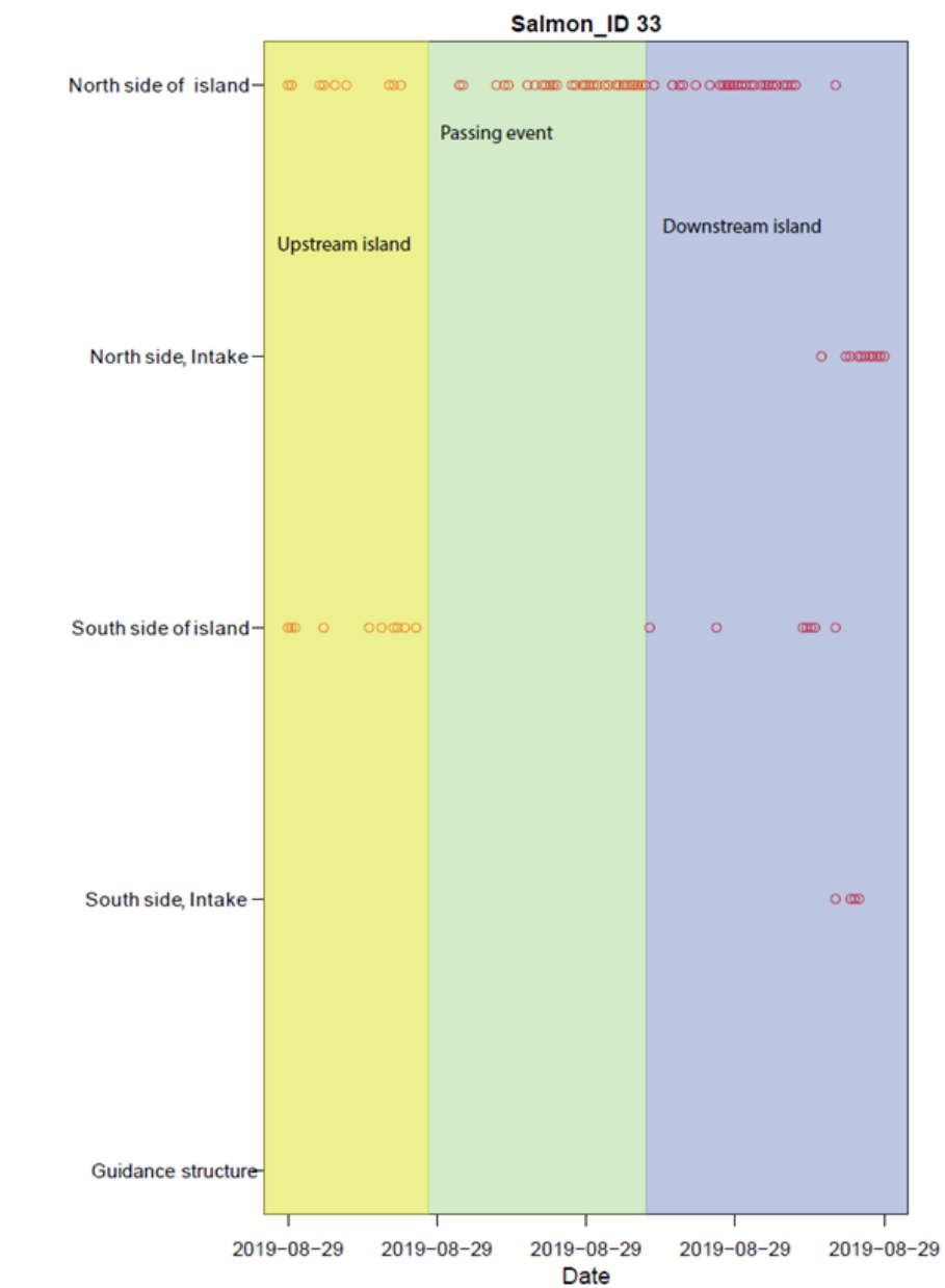
Example of visually determining which side of the island a fish passed, in a plot created in R with the package Glatos. Red dots represent registrations at a receiver
