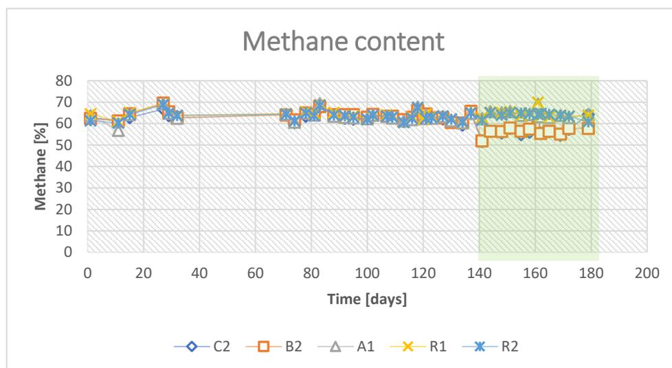
Figure 18. The methane content in the produced biogas from reactors C2, B2, A1, R1 and R2. The green field illustrates the time when the total ammonium-nitrogen was increased.
