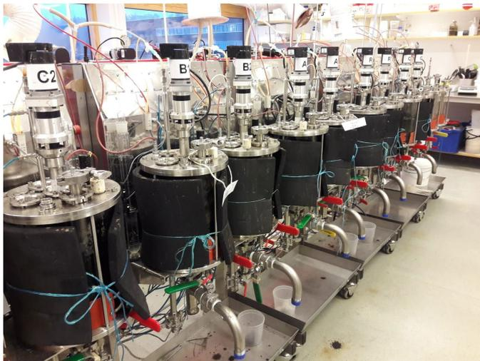
*Figure 5.* The continuously stirred reactors that were used in this study.
