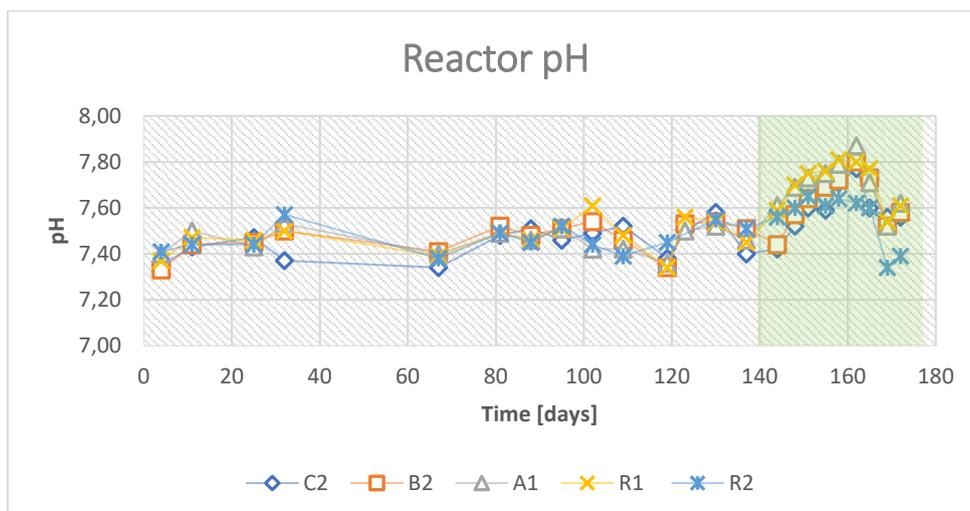
Figure 17. The pH levels in the investigated reactors. The green field illustrates the time when the total ammonium-nitrogen was increased.
