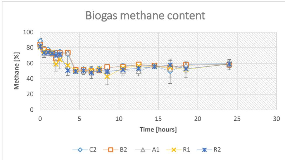
Figure 8. The methane content of the produced biogas in reactor C2, B2, A1, R1 and R2.
