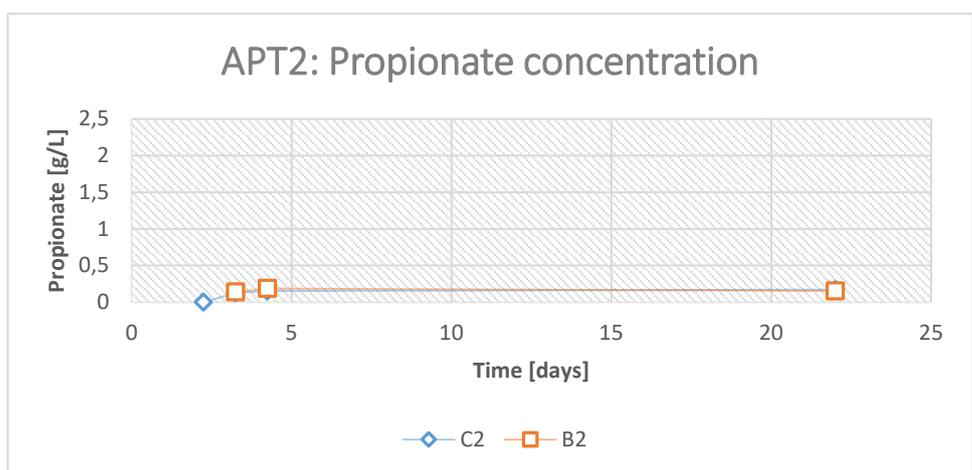
Figure 14. The concentration of propionate in reactors C2 and B2 after being pulsed with 5.7 ml acetic acid after 0 hours and fed with substrate after 1.25 hours.
