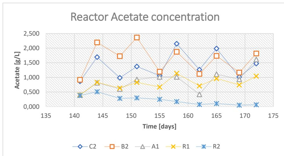
Figure 21. The acetate concentration in reactors C2, B2, A1, R1 and R2 during day 141 to 172. Reactors C2, B2, A1 and R1 were subjected to an increase in ammonia and reactor C2 and B2 were in addition pulsed with acetic acid.
