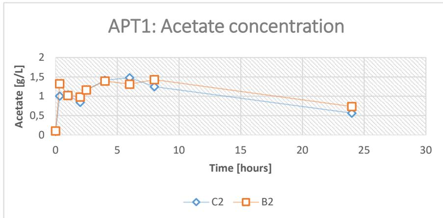
Figure 10. The concentrations of acetate in reactors C2 and B2 after being pulsed with 5.7 ml acetic acid after 0 hours and fed with substrate after 2 hours during APT1 (acetic acid pulsing test 1).
