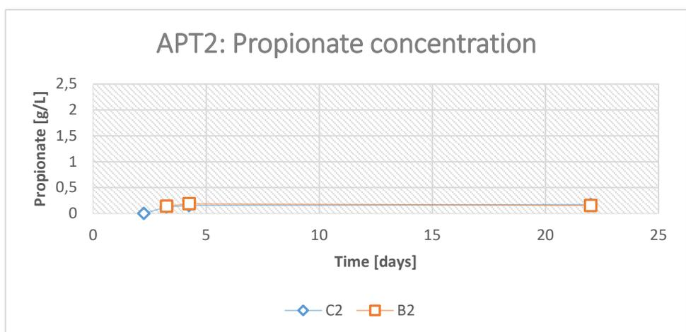
Figure 14. The concentration of propionate in reactors C2 and B2 after being pulsed with 5.7 ml acetic acid after 0 hours and fed with substrate after 1.25 hours.
