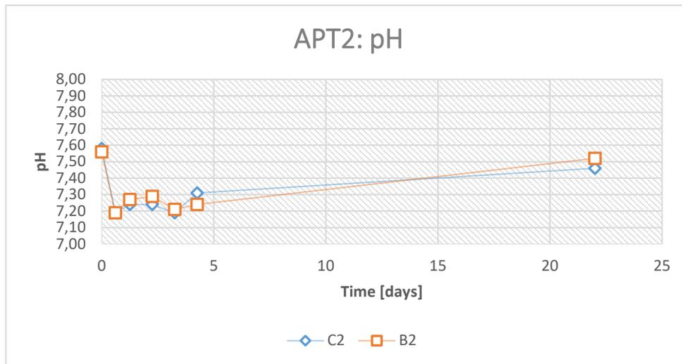
Figure 15. The pH levels for reactor C2 and B2 during the second acetic acid pulsing test.
