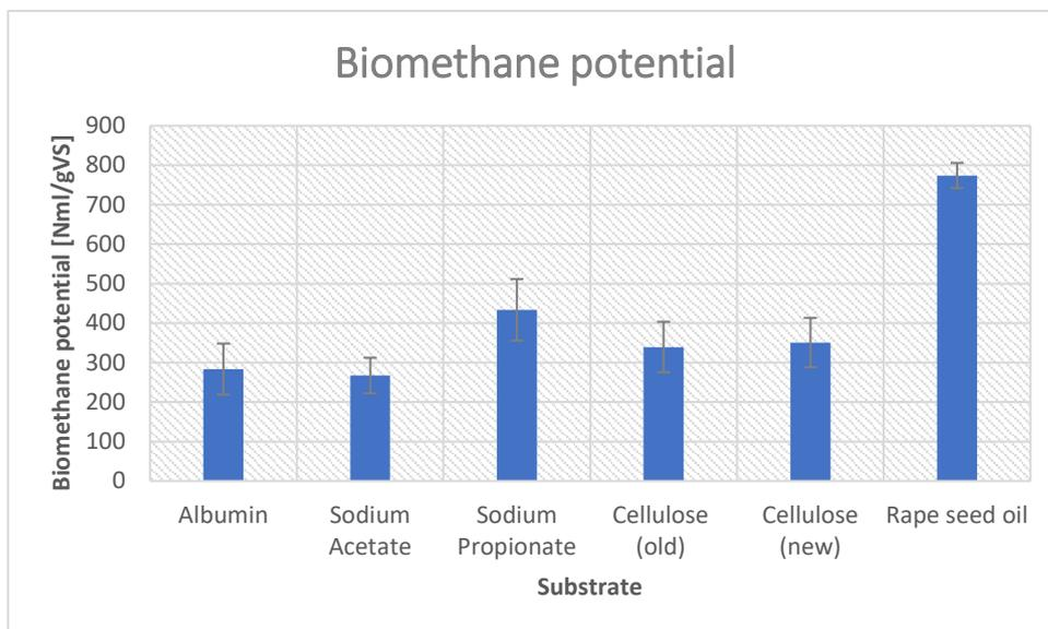
Figure 9. The biomethane potential from the substrates; albumin, sodium acetate, sodium propionate, two batches of cellulose (one older than the other but no other differences) and rape seed oil.
