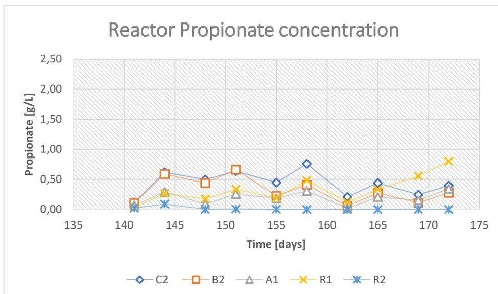
Figure 22. The propionate concentration in reactors C2, B2, A1, R1 and R2 during day 141 to 172. Reactors C2, B2, A1 and R1 were subjected to an increase in ammonia and reactor C2 and B2 were in addition pulsed with acetic acid.
