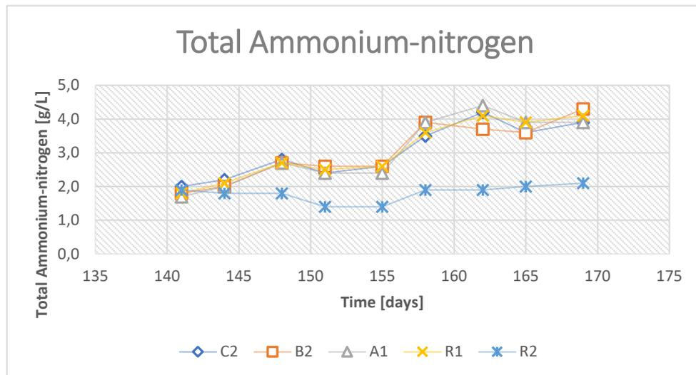
Figure 16. The total ammonium-nitrogen concentrations for reactors C2, B2, A1, R1 and R2 during the increased ammonia test (days 140-169).
