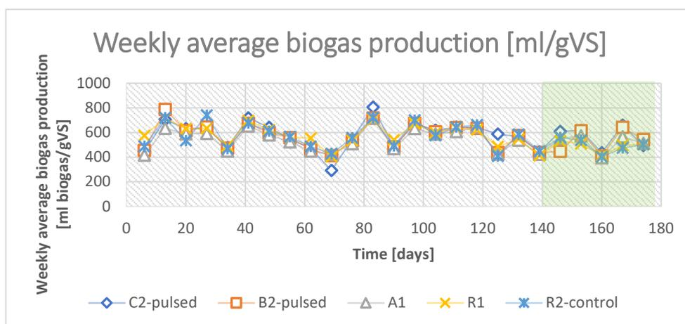
Figure 18. The weekly average biogas production for reactors C2, B2, A1, R1 and R2. The green field illustrates the time when the total ammonium-nitrogen was increased.
