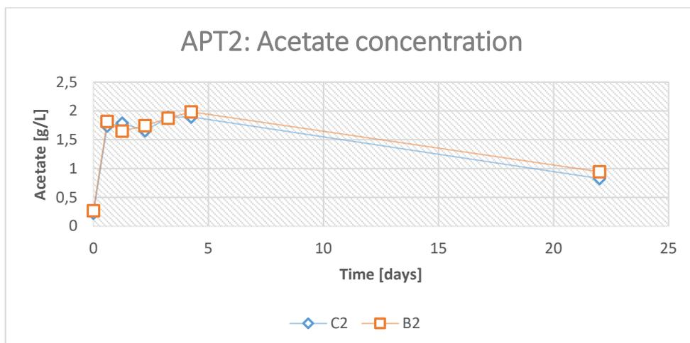
Figure 13. The concentration of acetate in reactors C2 and B2 after being pulsed with 5.7 ml acetic acid after 0 hours and fed with substrate after 1.25 hours.
