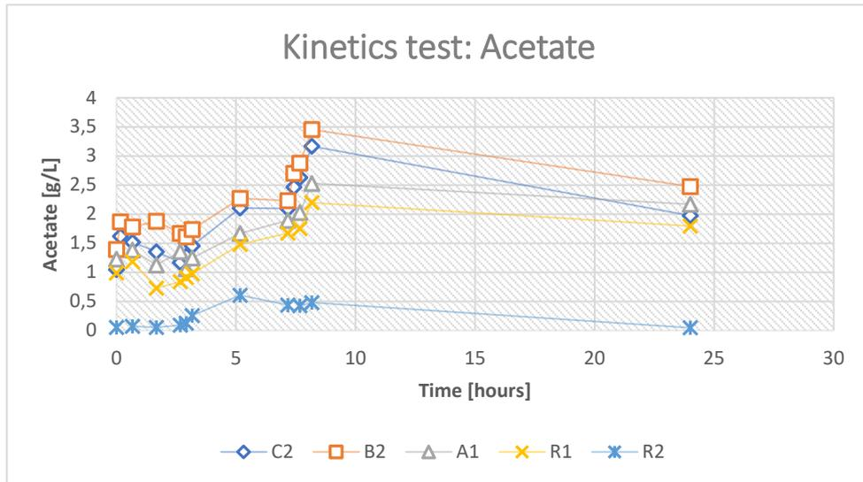
Figure 23. The figure shows the acetate concentration in reactors C2, B2, A1, R1 and R2 during the kinetics test.
