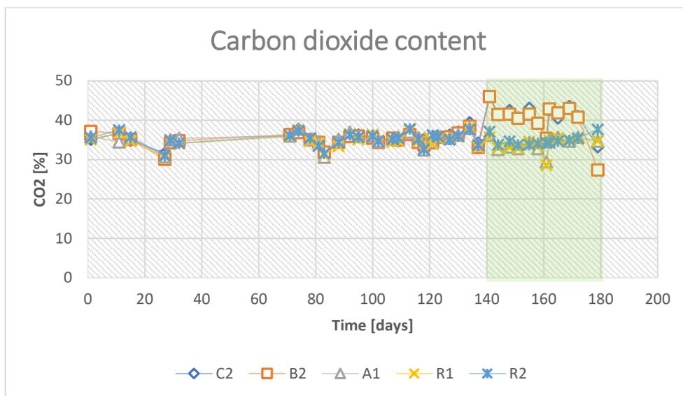
Figure 19. The carbon dioxide content in the produced biogas from reactors C2, B2, A1, R1 and R2. The green field illustrates the time when the total ammonium-nitrogen was increased.
