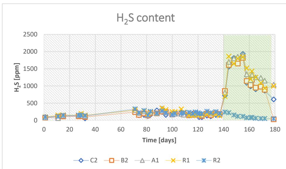
Figure 20. The  $H_2S$  content in the produced biogas from reactors C2, B2, A1, R1 and R2.
