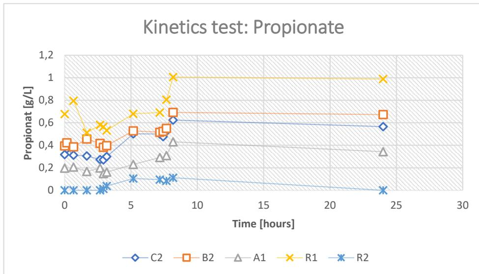
Figure 24. The figure shows the propionate concentration in reactors C2, B2, A1, R1 and R2 during the kinetics test.
