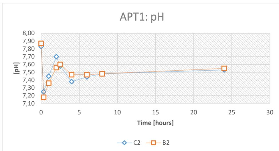
Figure 12. Variation of pH-level during the 24-hour test period of APT1 (acetic acid pulsing test 1), where reactors C2 and B2 were pulsed with 5.7 ml acetic acid after 0 hours and fed with substrate after 2 hours.
