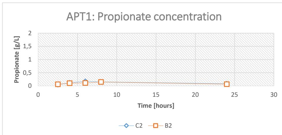
Figure 11. The concentration of propionate in reactors C2 and B2 after being pulsed with 5.7 ml acetic acid after 0 hours and fed with substrate after 2 hours during APT1 (acetic acid pulsing test 1).
