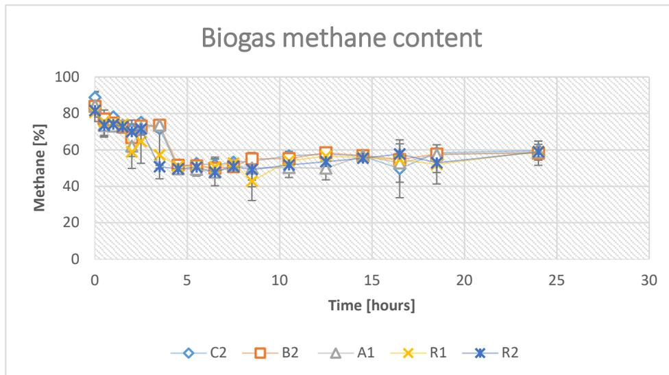
Figure 8. The methane content of the produced biogas in reactor C2, B2, A1, R1 and R2.
