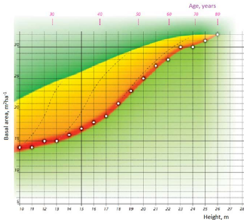
Figure 14. Model for thinning in pure spruce stands on fertile soil types. (LVM, 2008) Green area – zone where thinning is necessary, yellow area – optimal basal area, red area – critical basal area.
