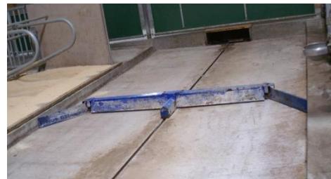
Figure 5. Automatic scraper on solid floor. Photo: Christer Bergsten
