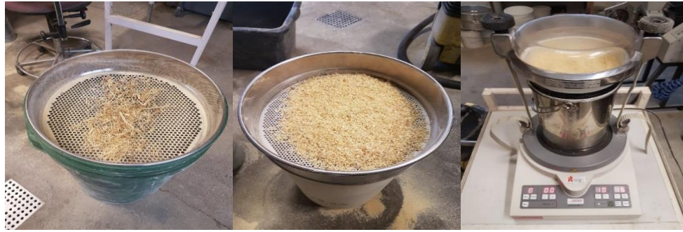
Figure 5. Left: Sieve size 8.00 mm. Centre: Sieve size 3.15 mm. Right: Sieve table (Photo: Tobias Holdo)
