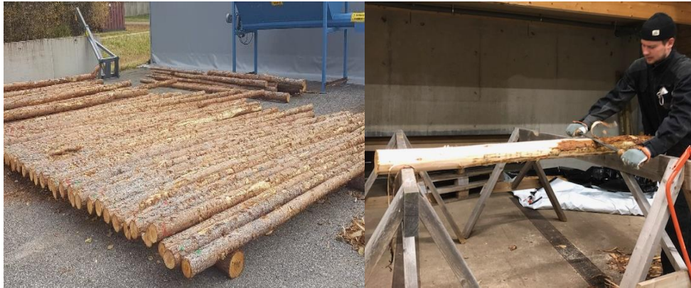
Figure 2. Left: Experimental logs during storage. Right: Manual debarking of logs. (Photo: Atanu kumar das)
