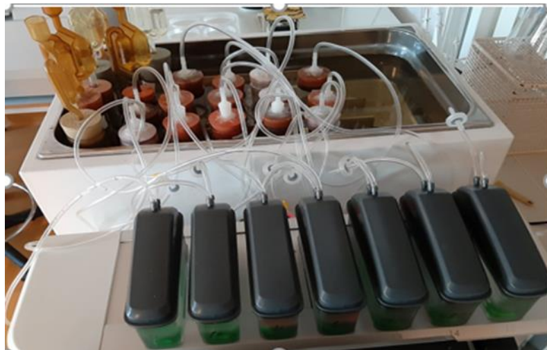
Figure 4. An image of the experimental setup. The gas measurement unit of Gas Endeavour (Bioprocess Control AB, Lund, Sweden) was used to record the gas production.
