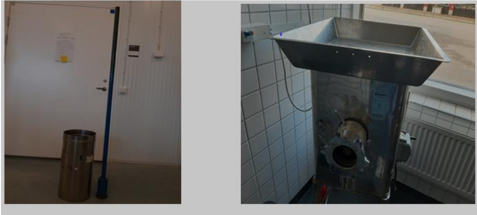
Figure 1. The metal rod and container used for mild mechanical treatment and the meat mincer used for harsh mechanical treatment.
