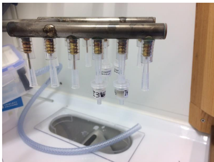
Figure A2: Nitrogen flow distributor used to gently dry attached TIMFIE SPE cartridges.
