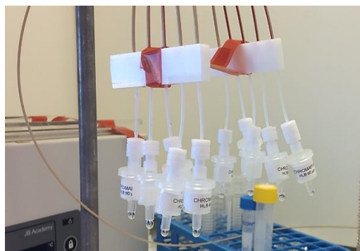
Figure A1: Simultaneous conditioning of HLB cartridges on a flow distributor.
