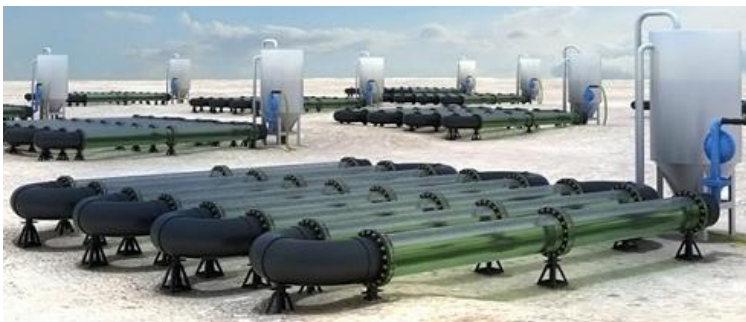
Tubular photobioreactor outside system (Fredin, 2009)
