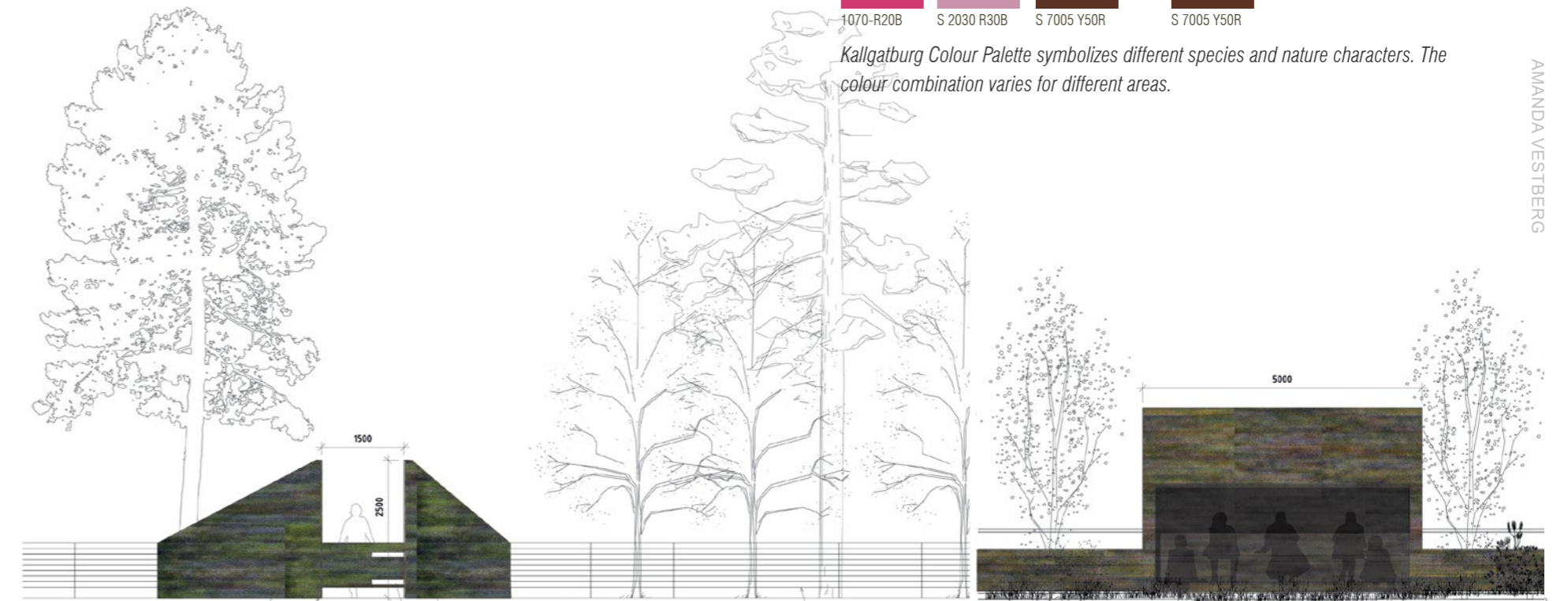
A portico marks the shift between different nature characters within Kallgatburg. The Porticos function is to clarify the areas nature characters, provide information for the specific spot and create a more accessible or passable fence passage.
