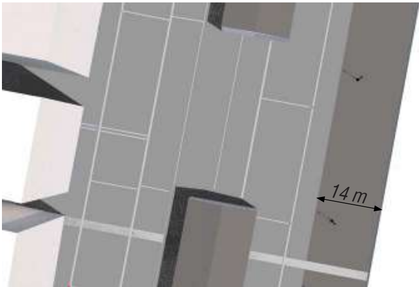
Figure 29. Conceptual image of pipeline outlines below Skeppsbron. Note the pipe line free zone.
