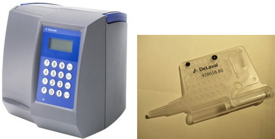
Picture 3: The Delaval's somatic cell counter DCC and the cassette used to draw the milk up in capillary tubes.
