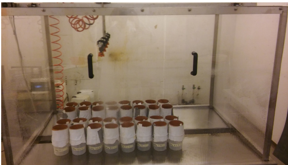
Figur 11. 32 aggregatprov i regnsimulatoren.
