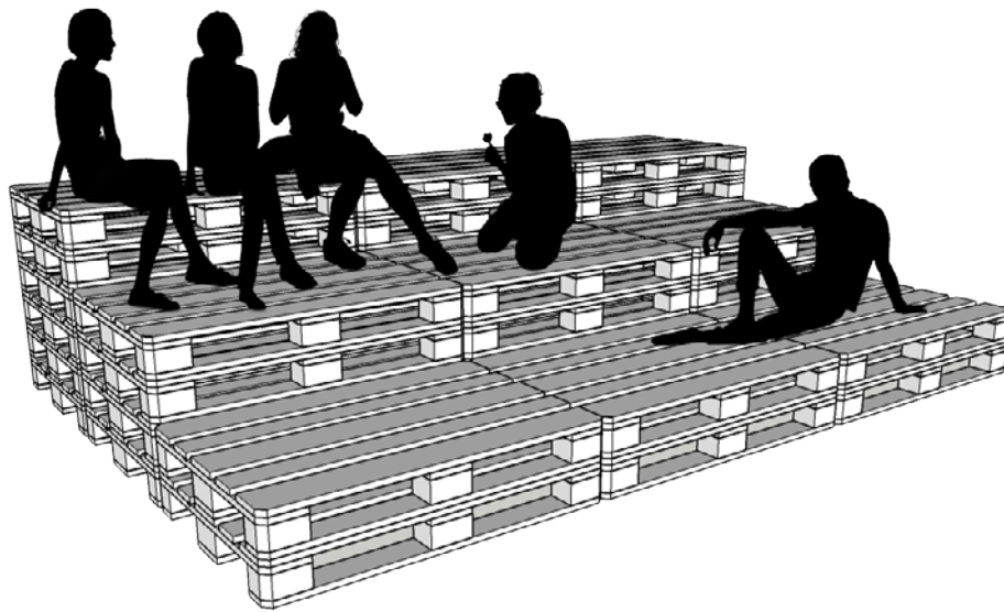
Figure 7.13 Diagram showing how pallets could be formed into a stand
