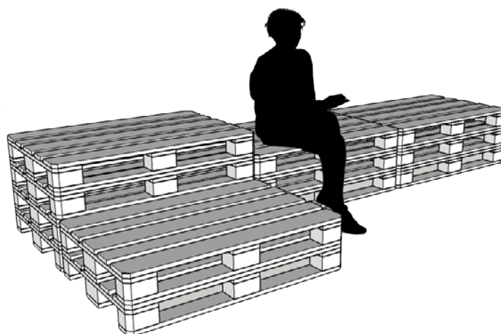
Figure 7.15 Diagram showing how pallets could be formed into a bench
