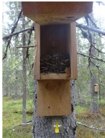
Figure 2. Nest box with two attached temperature loggers, one directly under, and one placed inside the nest box.
