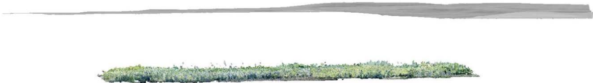
Figure 5. One of the point clouds generated visualized in QTModeler with a DEM from the land survey. The point cloud (the lower part) is not in line with the DEM from the land survey (the upper part).
