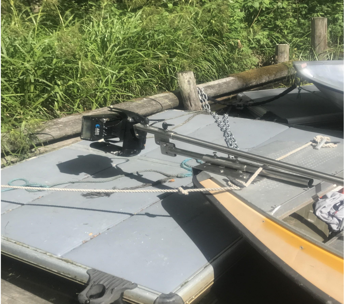
Figure 5. Photo showing the setup of the ARIS device in the front of the boat. When recording, the device was lowered into the water by turning the long metal arm into a vertical position. The ARIS could then be turned using the ARIS rotator AR2, seen on the picture as a shackle to which the metal arm is attached
