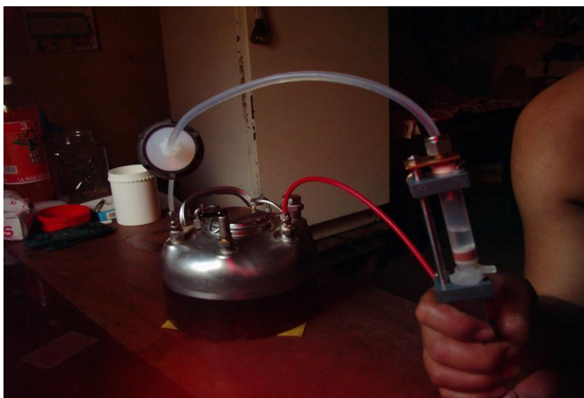
Photo 11. The SPE-technique. The water sample is forced through the SPE-cartridges with air pressure. The pressure is created in the sampling vessel with a bicycle pump due to vacuum in the vacuum chamber. First the water passes through a filter (Whatman GFF glass microfibre, 47 mm diameter) that collects the particles in the sample and then through the cartridges. If needed, the filter can be changed. The water that passes through the cartridge is then collected and the volume measured (Kylin 2007).
