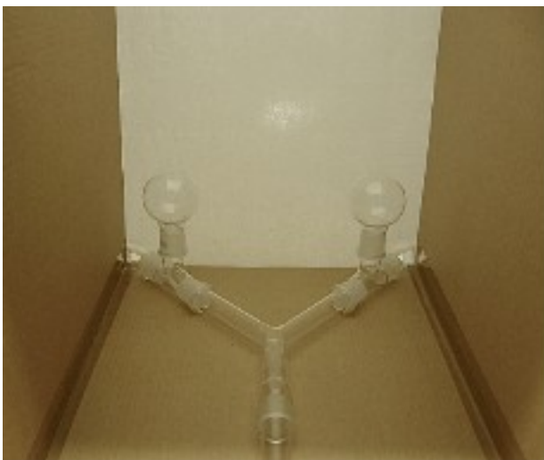
Figure 2. The female y-tube olfactometer bioassay setup. The male setup did not have the insect trapping bulbs.
