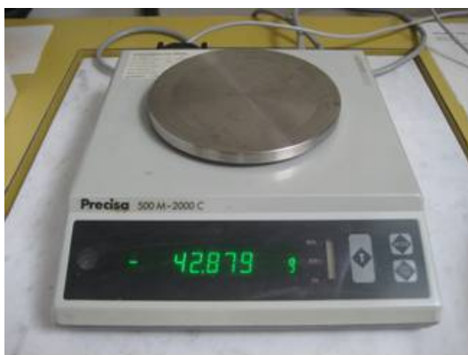
Figure 20. Electronic scale used to measure the dry weight of cuttings, shoots, roots and leaves. Photo: Teresa Brage Tuñón
