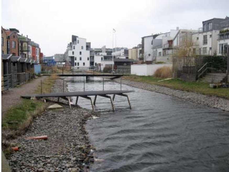
A canal in Bo01 that lets the sea water fluctuate and also receives storm water from the residential area. The canal is an important element in the design. (Photo: S. Rytter)
