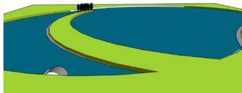
Figure no 12 A land strip forces the contaminated water to flow through the whole pond.
