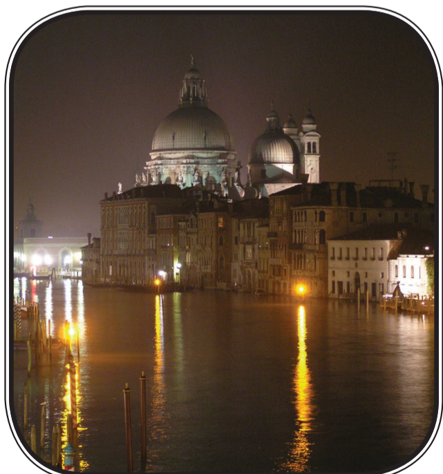
Glare from floodlights affects the light distribution. Further there are differences in light colour.
