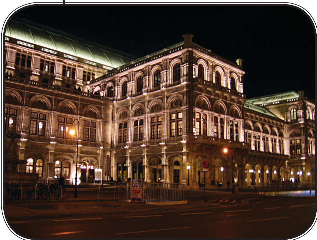
Accent lighting of the Opera house in Vienna, Austria. A different light source with warmer colour temperature have been used for the lighting of the road.
