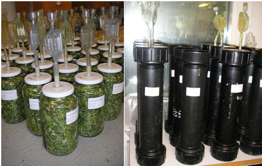
Figure 2: Glass silos (left) and PVC silos (right) used in the ensiling study
