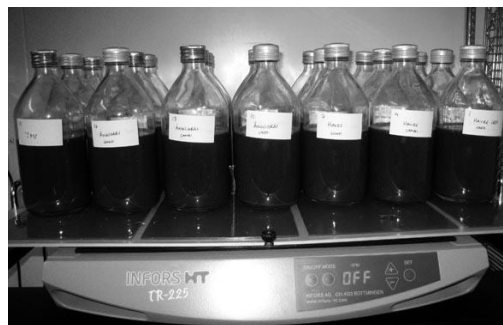
Figure 4. The bottles in the batch experiment during incubation in a constant temperature room on a shake table.
