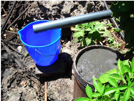
Fig. 6. Water sample collection in staff kitchen, with the simple filter filled with sludge in the right-hand corner.
