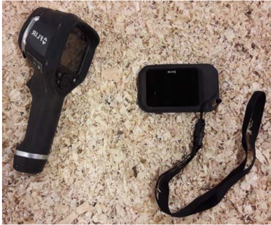
Figure 6: Shows the IR cameras; FLIR E8 and FLIR C2, in that order.
