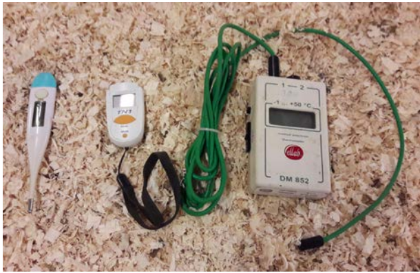
Figure 4: Shows the rectal thermometer (Microlife AG, model MT20RA), the IR meter (TN1) and the skin temperature meter (DM852), in that order.
