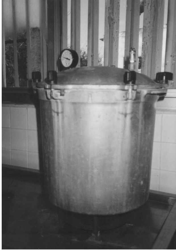
Picture 9: All test tubes and agar was sterilised in this pressure cooker.
