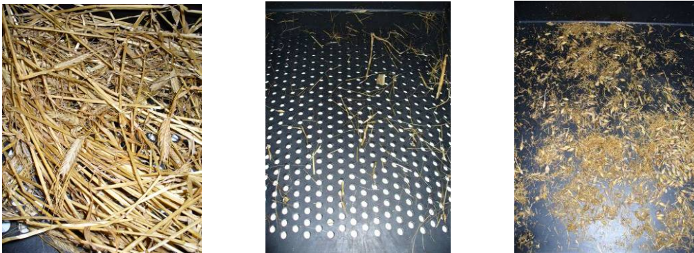
Figure 17. Long silage at dough stage of maturity after sieving. Upper and lower sieve and bottom pan are shown from left to right.
