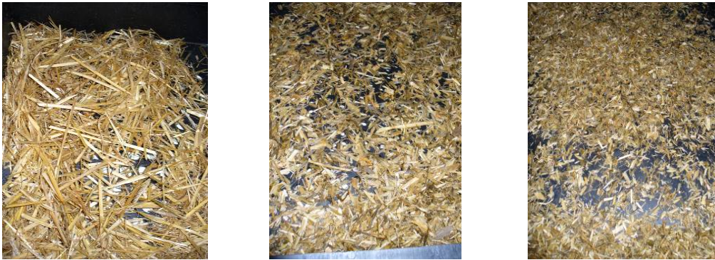
Figure 16. Chopped silage at heading stage of maturity after sieving. Upper and lower sieve and bottom pan are shown from left to right.
