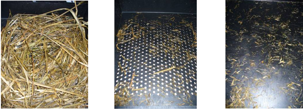
Figure 15. Long silage at heading stage of maturity after sieving. Upper and lower sieve and bottom pan are shown from left to right.
