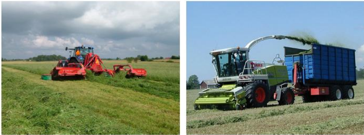
Figure 7. A mower-conditioner with nominal width of 9m (left) and a 40m 3 container pulled by a Claas Jaguar precision chopper in the ley field (right) (Vågström, 2005, p. 6).
