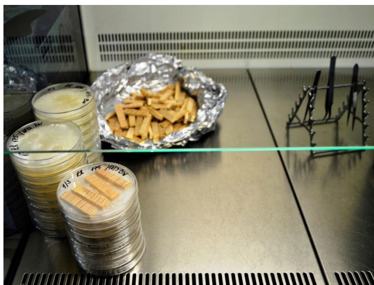
Figure 2. Long wood block application on Petri dishes fully colonized by H. parviporum .
