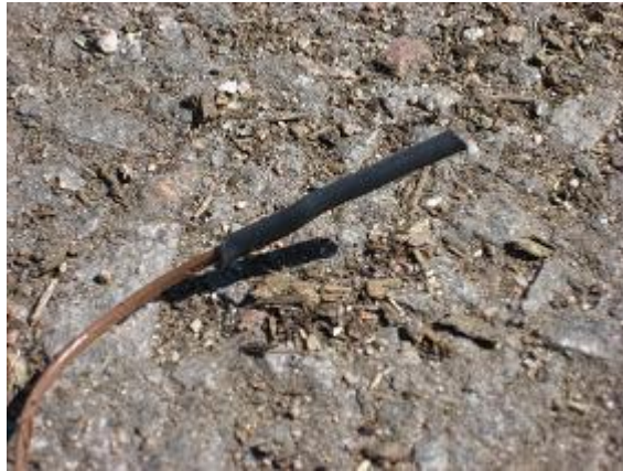
Figure 4.3, Thermocouple with measuring point covered with shrinking tubing
