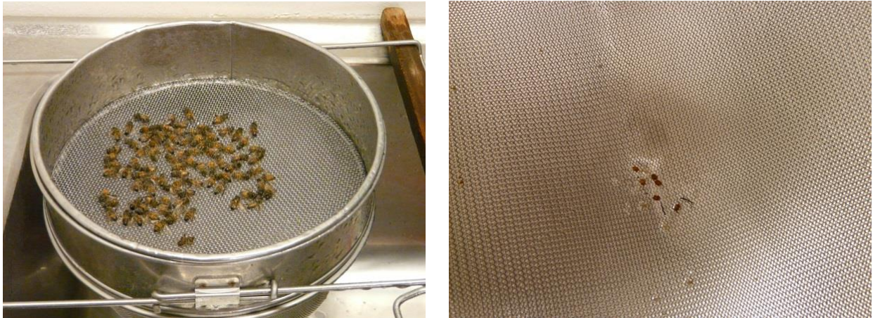
Figure 8. Double sieve with different aperture widths including a sample of bees (left, Photo: Julia Goss) and mites collected in the sieve after washing (right, Photo: Julia Goss).
