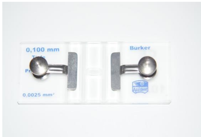
Figure 10. Haemocytometer model Bürker with 0.1 mm depth (Photo: Julia Goss).
