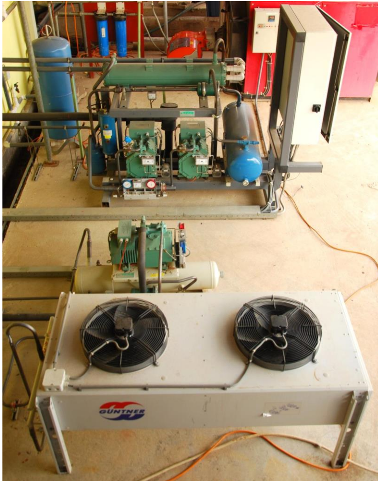
Figure 4.8: Bitzer tandem 2*24.6 A (water cooled) atop and Bitzer 1*15.9 A (air cooled)
