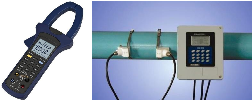
Figure 6.1: Multimeter with current clamp and ultrasonic heat energy meter with flow transducers
