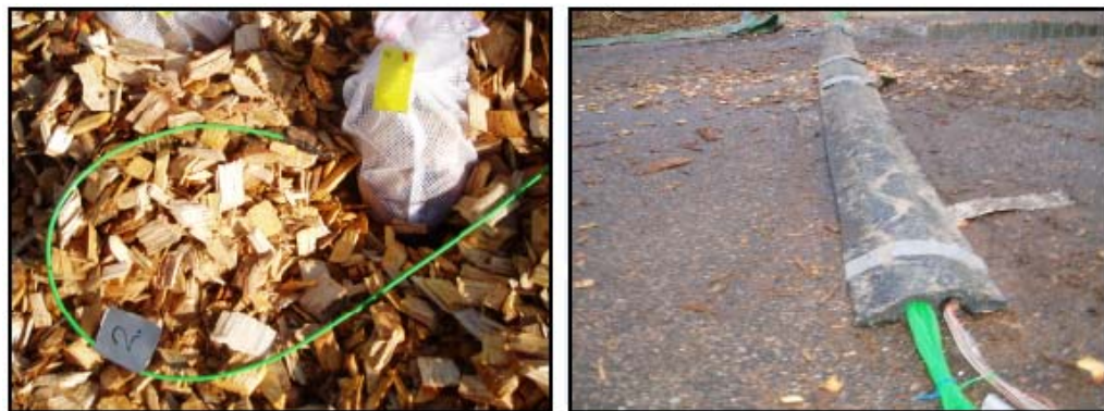
Figure 5.4, The left picture: A thermocouple and a sample bag filled with chips. The right picture: The thermocouples and the rubber cable protector.
