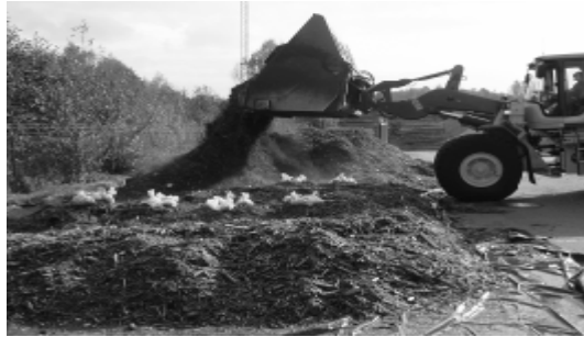
Figure 5.5 , The building of the second layer of the waste wood piles with sample bags at the sampling points.
