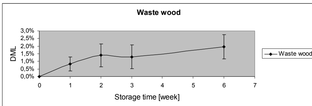
Figure 6.7 , Accumulated, dry matter losses (DML % dry weight basis) for each cross section based on an average from the 28 sample bags at the seven measuring points. A 95% confidence interval for each section is also included.
