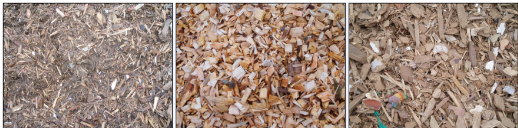
Figure 5.1 , The left picture: Waste wood chips for the six weeks storage trial. The middle picture: Stem wood chips for the six weeks storage trial. The right picture: Waste wood chips for the four days storage on ground heating surface trial.
